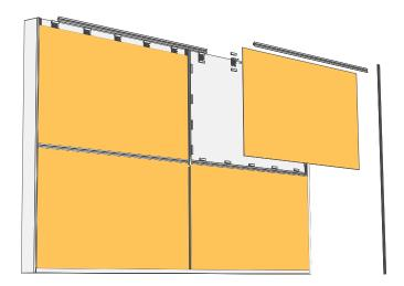
No additional off-site fabrication required. Panels are cut to fit on site and secured using a patented process, saving time and money.
