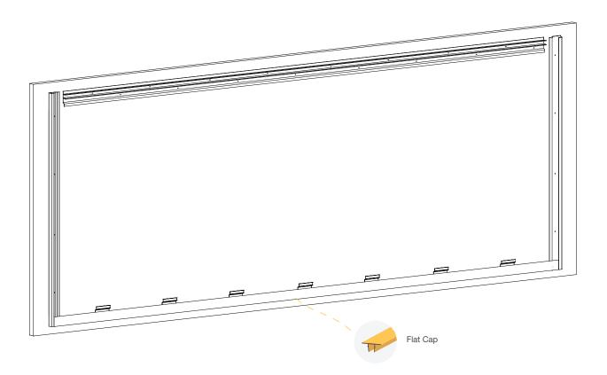
The flat cap needs to be cut to size and engaged using an AL13 SLED before the first row of v-line plank may be installed. A properly fit cap should tuck under both verticals leaving approx. a 1/8" gap on either side to allow for contraction and expansion. If a butt joint is required due to the length of the flat cap exceeding 12', the butt joint MUST occur on a shared back plate segment.
