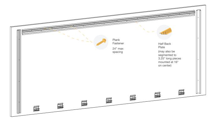
The final perimeter extrusion to be attached is the upper horizontal back plate.
