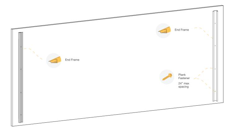
The vertical perimeter extrusions are normally the first extrusions to be fixed to the wall. The building wrap/envelope must be complete to spec before anything goes on the wall. Layout end frame extrusions according to the desired location. Ensure frames are level and plumb before fastening.
