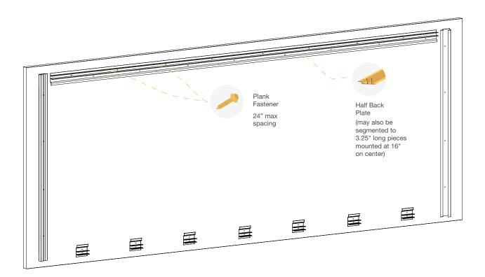
The final perimeter extrusion to be attached is the upper horizontal back plate.
