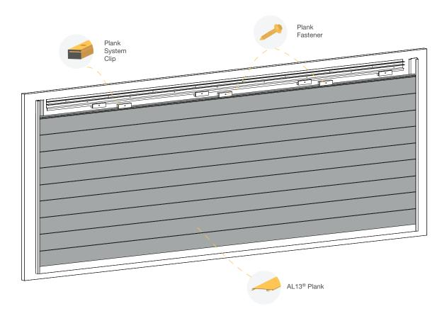
The final or top row to be installed may require the plank to be ripped to width by a table saw to its appropriate dimension. Due to this, the top rows installation may vary from the regular installation.
