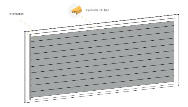
To secure the final row, a perimeter flat cap must be cut to length to fit behind the vertical frame extrusions. A proper fit should allow for a 1/8" gap on either side to allow for contraction and expansion. The perimeter flat cap should be hammered in place using an AL13® SLED with a rubber mallet.
