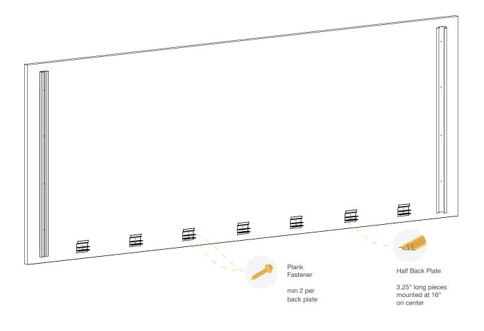
This will establish the horizontal datum - and will be a reference to subsequent extrusions - so it is important that it is mounted level.
