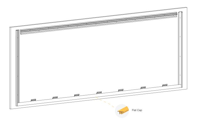
The flat cap needs to be cut to size and engaged using an AL13° SLED before the first row of the planks may be installed. A properly cut cap should tuck under both verticals leaving approx. a 1/8" gap on either side to allow for contraction and expansion. If a butt joint is required due to the length of the flat cap exceeding 12', the butt joint MUST occur on a shared back plate segment.
