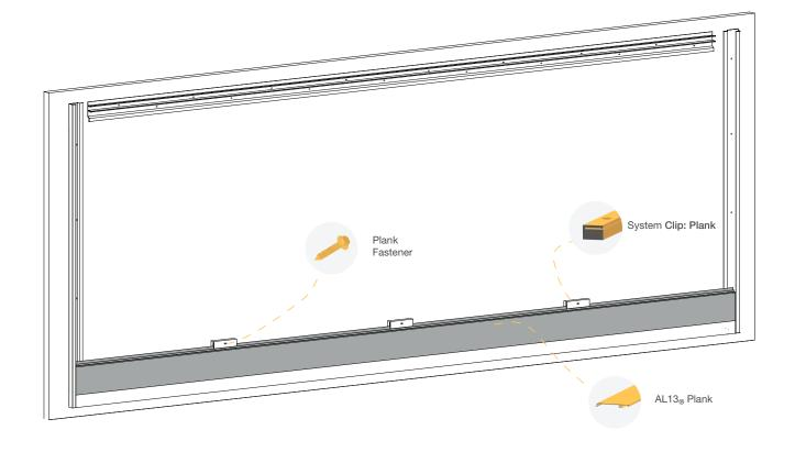
A properly cut plank should have a 1/8" gap from the components on either side to allow for thermal expansion.
