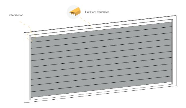
To secure the final row, a Flat Cap: Perimeter must be cut to length to fit behind the vertical frame extrusions. A proper fit should allow for a 1/8" gap on either side to allow for contraction and expansion. The perimeter flat cap should be hammered in place using an  $AL13_{\odot}$  SLED with a rubber mallet.
