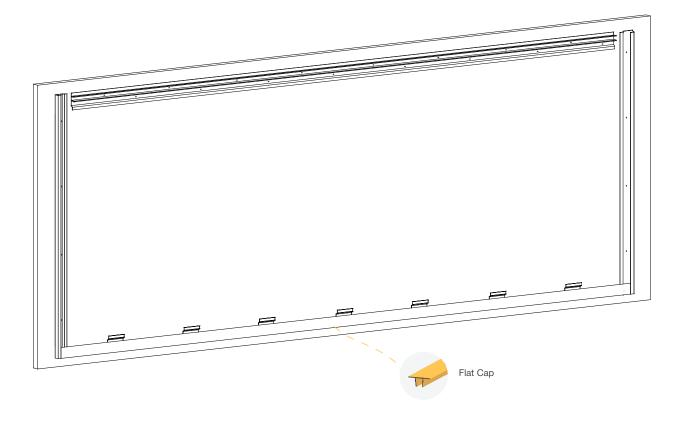
The flat cap needs to be cut to size and engaged using an AL13 $_{\circ}$  SLED before the first row of v-line plank may be installed. A properly fit cap should tuck under both verticals leaving approx. a 1/8" gap on either side to allow for contraction and expansion. If a butt joint is required due to the length of the flat cap exceeding 12', the butt joint MUST occur on a shared back plate segment.
