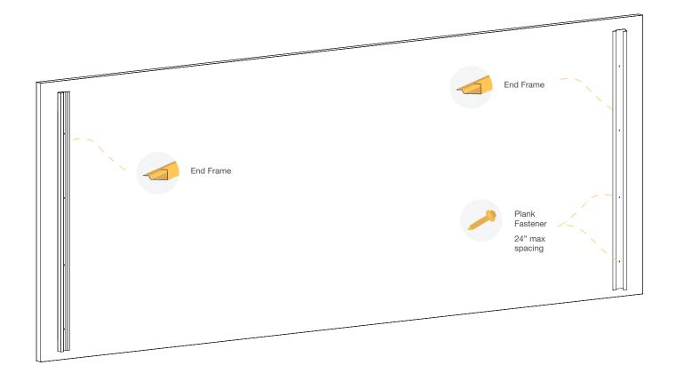
The vertical perimeter extrusions are normally the first extrusions to be fixed to the wall. The building wrap/envelope must be complete to spec before anything goes on the wall. Layout end frame extrusions according to the desired location. Ensure frames are level and plumb before fastening.
