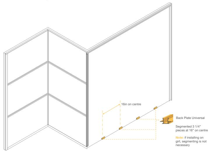
The AL13® Panel System is a rain screen system that does not require any strapping.
