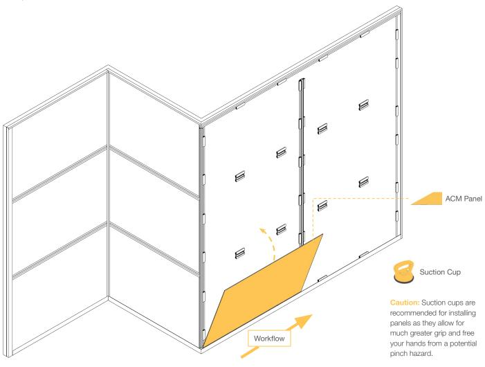
**Step 1** - position panel on its long edge, lift it up and place in position.
