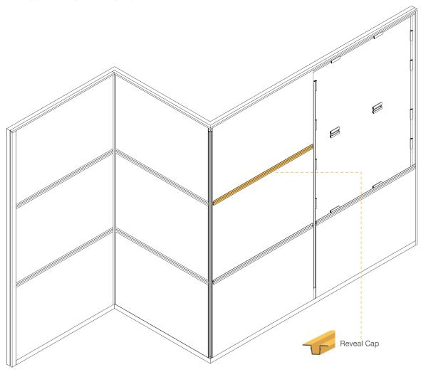
After the ACM Panels have been shifted into the correct position, the horizontal top cap will secure the panels in place. Once the top cap is cut to the appropriate length, it should be placed, one end first, into place, with each end under the tabs of the horizontal End Frames.
