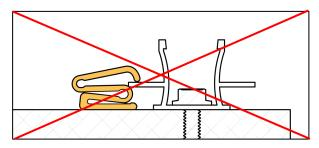
Note that the System Clip Compressible presses up against the panels, hence the majority of its body needs to rest towards the panel.
