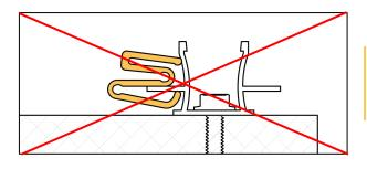
This incorrect, upside-down installation will also not provide the correct fit between the framing and the ACM panels.
