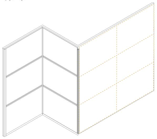
Using the chosen layout, determine the best suited datum - or starting point - shown here as the lower left corner. Lay out the panel grid using chalk lines (or similar) from the datum point, ensuring that all lines are plumb or level. These lines are to indicate the locations of the extruded frame components that will secure and frame the ACM panel.
