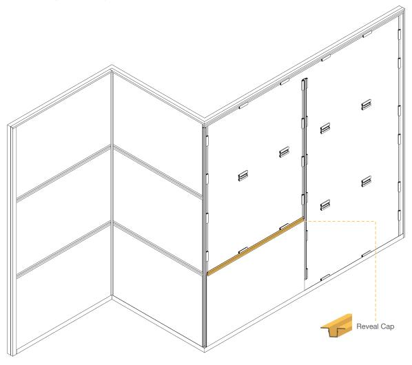
After the ACM Panel has been shifted into the correct position you must securely fasten it in place with a top cap. The top cap is the second part of the two-part Panel Frame Assembly which is snapped into place with a rubber mallet and the AL13® SLED.
