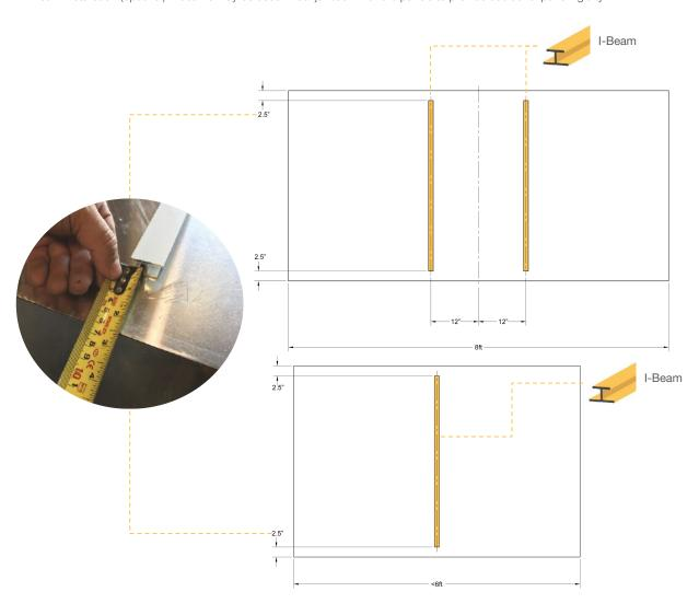
Step 1 - Cut I-beams to fit.
