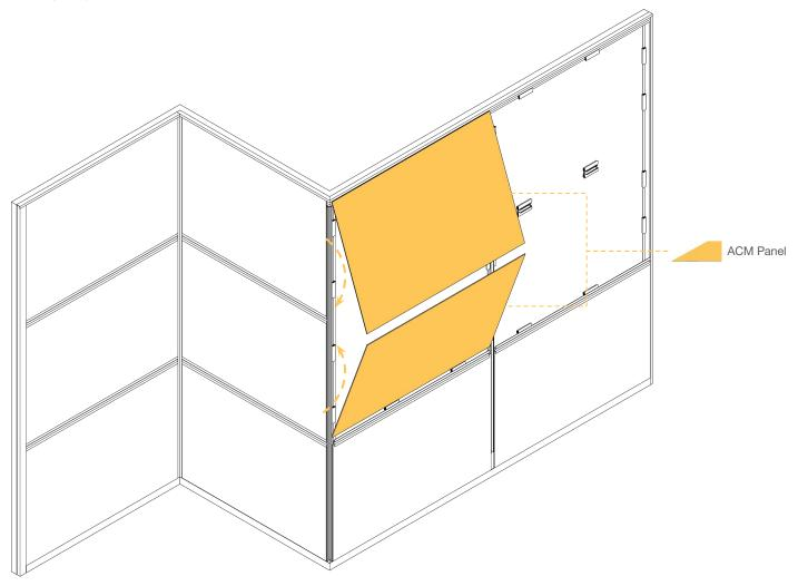
The top two panels in a column must be installed simultaneously. Since the top of the wall terminates under the horizontal End Frame, it would be impossible to place the upper panel if the below top cap was already secured.
