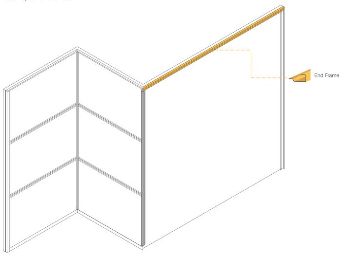
The upper End Frame is next to be measured and cut-to-size. A double mitre could be required if the vertical End Frames are mitered at 45 degrees (as outlined in the previous step).
