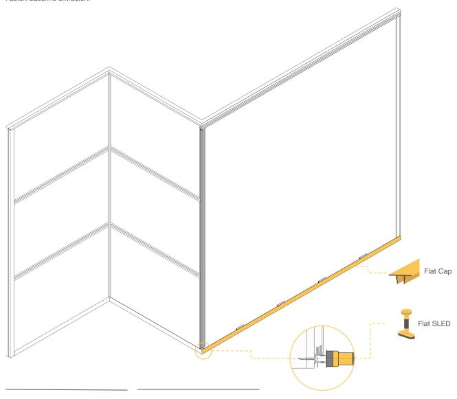
Measure and cut the bottom horizontal top cap. A proper fit will ensure that either end may be tucked into the vertical end frames, leaving a minimum 1/8" gap to allow for proper contraction and expansion of the extrusion.
