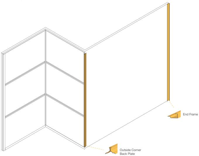
Measure and cut the vertical End Frames according to the marked grid lines. If the top of the vertical End Frame is to meet another horizontal End Frame at 90 degrees, a 45-degree mitre cut is to be made on both parts to complete the angle. This will eliminate the need to notch extrusions. If the wall is to be finished with a half back plate and perimeter cap, the 45-degree mitre is not necessary, as the horizontal cap will tuck behind the vertical end frames.
