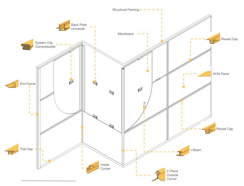
The backplates and various caps use an interference fit and require an impact to engage the two components. Ensure that the substrate is solid enough to sustain this impact.
