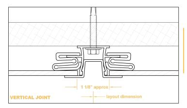
Standard panel size is 4 ft x 8 ft (1220 mm x 2440 mm). Do not use these dimensions for determining layout lines, adequate space must be left between panels for extrusions.
