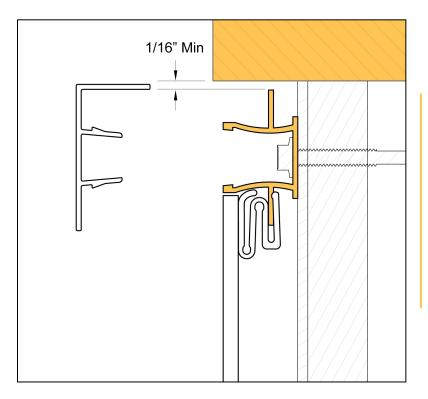
Leave a minimum of 1/16" gap between the edge of a perimeter (e.g., windows, doors, bump-outs) and the Back Plate Universal.
