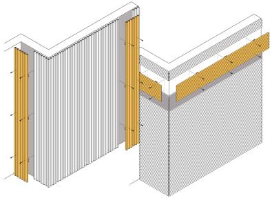
The AL13<sub>®</sub> batten system provides the traditional look of wood and durability of metal on walls and ceilings.
