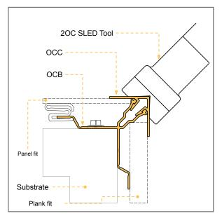
The **2-Piece Outside Corner (20C)** provides a method to terminate a wall assembly in situations where using the standard Outside Corner would make terminating the wall difficult. The 20C works with both the AL13 Panel System® and AL13 Plank System® and comprises two components: **OCB** (back plate) and the **OCC** (cap).
