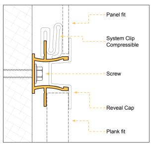
The **Back Plate: Universal (BPU)** anchors the AL13 Panel System® and AL13 Plank System® on to the wall substrate. It is used for both around the perimeter and along the wall, and is used at full length or as 3.25" segments. The BPU is compatible with the following top caps:
