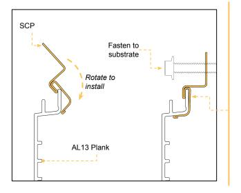
The **System Clip: Plank** provides an interface between AL13® Planks and the substrate. They secure the planks to the wall with an AL13®approved fastener appropriate for the substrate. The SCP can only be engaged in one position correctly.
