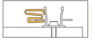
Install the system clip correctly by ensuring the Backplate is inserted into the engaging slot as shown.
