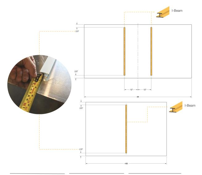
**Step 1** - Cut I-beams to fit. Appropriate sizing should be offset from either edge of the panel 2 1/2". Full 4 ft × 8 ft panels will require 2 I-beams set back 12" from the centre. Panels 6' or below only require 1 I-beam, running in the narrow direction, at the center of the panel.
