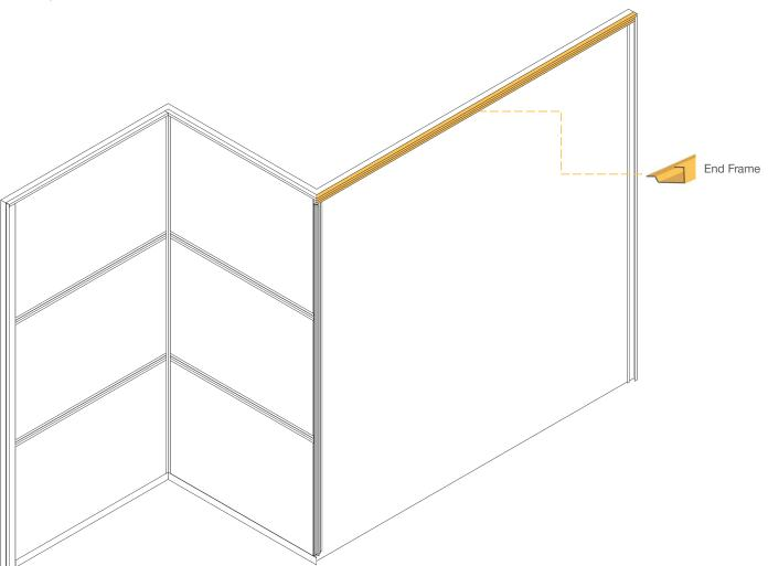
The upper End Frame is next to be measured and cut-to-size. A double mitre could be required if the vertical End Frames are mitered at 45 degrees (as outlined in the previous step). If one length of the End Frame extrusion is not long enough to span the distance required, it is necessary to use a second piece and butt the two together. Take care in aligning joints so that they are flush, shim as needed.
