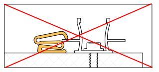
Note that the System Clip Compressible presses up against the panels, hence the majority of its body needs to rest towards the panel.
