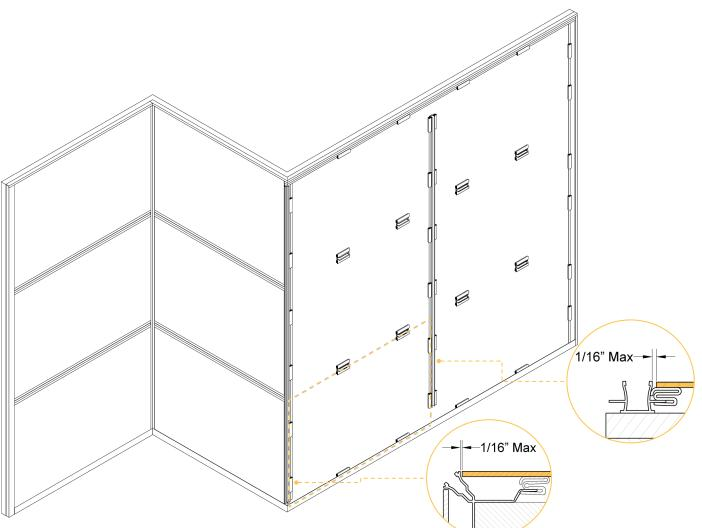
Once a panel is ready to be fit, it may be taken off the stack. Make sure not to drag sheets across, rather lift the sheet up off the stack, then away. Although the panels have a protective film applied from the factory, reckless panel handling may cause damage to the panel through the wrap. It is recommended that at least two persons carry one sheet. The protective film should be peeled back approximately 1" (25 mm) from the edges, but should remain on the panel otherwise.
