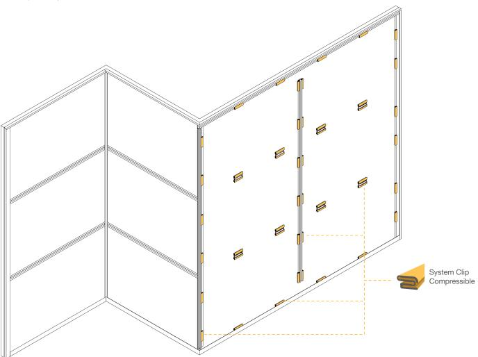
Once all extrusions have been installed it is time to attach system clips to all the extruded frame components. Systems clips act as spacers and are installed with the thin tab pointing towards the wall and the thicker portion facing away from the wall. System clips keep the panels tight to the frame without the need for adjustment.
