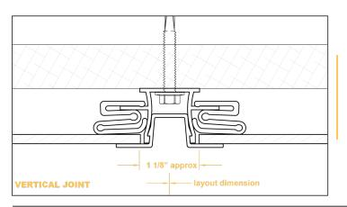
Standard panel size is 4 ft x 8 ft (1220 mm x 2440 mm). Do not use these dimensions for determining layout lines, adequate space must be left between panels for extrusions.
