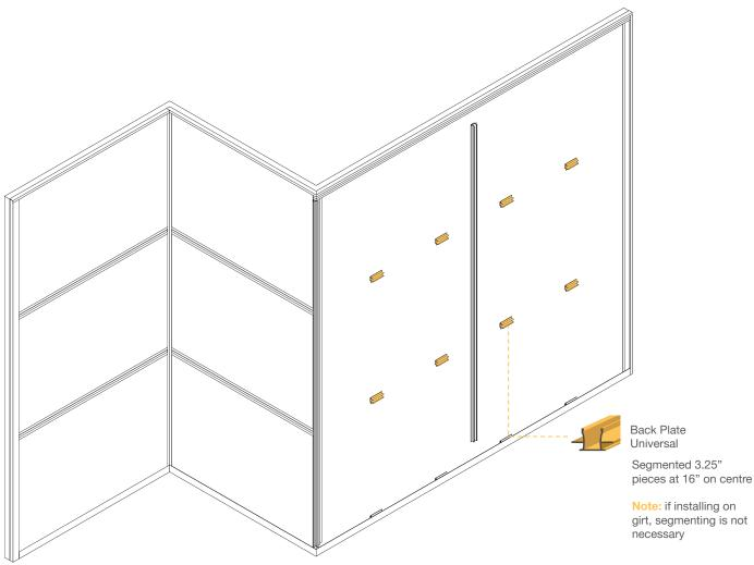
Measure and cut horizontal back plates in 3 1/4" segments and install them every 16" as per the layout. If you are fastening to a minimum of ½" ply or OSB sheeting, it is not necessary to fasten segments to a stud. It is recommended to pre-drill the holes in the segmented back plate pieces. This will prevent the small pieces from spinning while fastening which aides in eliminating the possibility of a cut hazzard.
