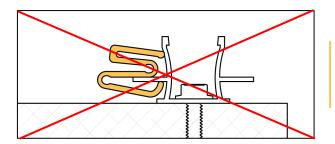
This incorrect, upside-down installation will also not provide the correct fit between the framing and the ACM panels.
