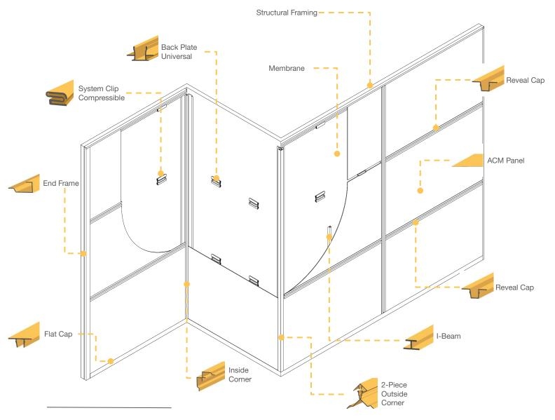
The backplates and various caps use an interference fit and require an impact to engage the two components. Ensure that the substrate is solid enough to sustain this impact.
