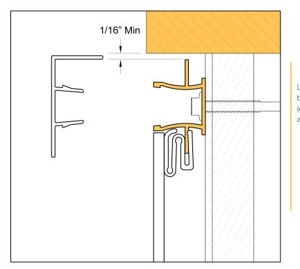
Leave a minimum of 1/16" gap between the edge of a perimeter (e.g., windows, doors, bump-outs) and the Back Plate Universal.
