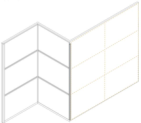
Using the chosen layout, determine the best suited datum - or starting point - shown here as the lower left corner. Lay out the panel grid using chalk lines (or similar) from the datum point, ensuring that all lines are plumb or level. These lines are to indicate the locations of the extruded frame components that will secure and frame the ACM panel.
