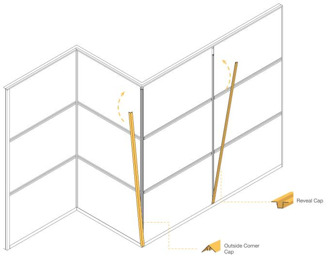
Once two adjacent columns of panels have been installed, the top cap may be installed. Once the top cap is cut to the appropriate length, it should be placed, bottom end first, into place with each end under the tabs of the horizontal End Frames. Once in the correct position it is to be hammered into place with a rubber mallet and AL13® SLED.
