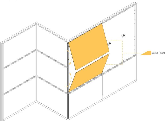
The top two panels in a column must be installed simultaneously. Since the top of the wall terminates under the horizontal End Frame, it would be impossible to place the upper panel if the below top cap was already secured. **Step 1** - Install lower panel and hold in place while second panel is fitted.
