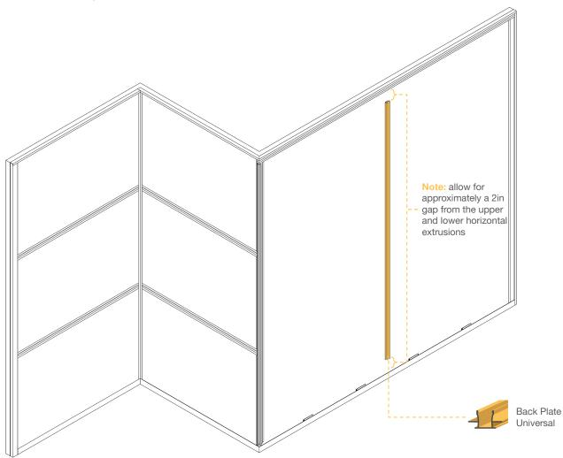
Measure and cut the vertical full back plate. Allow for approximately 2" gap from horizontal upper and lower extrusions to allow for proper top cap installation. Begin by fastening the top of the extrusion first (upper 3"), followed by the bottom (lower 3"), then the intermediate fasteners.
