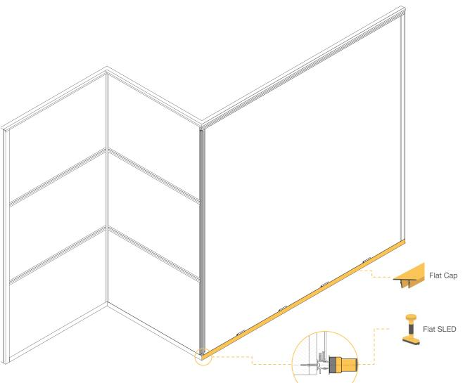
Measure and cut the bottom horizontal top cap. A proper fit will ensure that either end may be tucked into the vertical end frames, leaving a minimum 1/8" gap to allow for proper contraction and expansion of the extrusion. Engage the top cap into the segmented back plates using an AL13® SLED with a rubber mallet. It is imperative to only make contact where back plates are present so as not to damage or warp the top cap.
