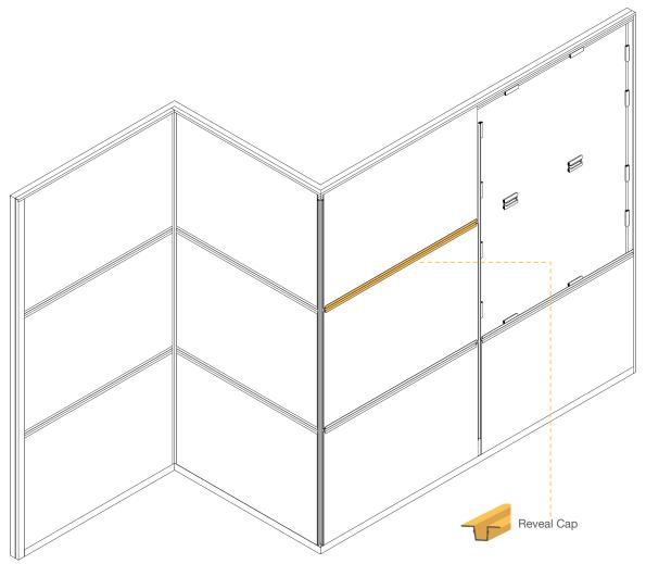
After the ACM Panels have been shifted into the correct position, the horizontal top cap will secure the panels in place. Once the top cap is cut to the appropriate length, it should be placed, one end first, into place, with each end under the tabs of the horizontal End Frames.
