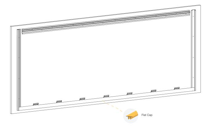
The flat cap needs to be cut to size and engaged using an AL13® SLED before the first row of the planks may be installed. A properly cut cap should tuck under both verticals leaving approx. a 1/8" gap on either side to allow for contraction and expansion. If a butt joint is required due to the length of the flat cap exceeding 12', the butt joint MUST occur on a shared back plate segment.
